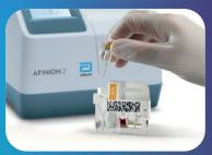
Place the test cartridge in the analyzer and close the lid. The processing starts automatically.
